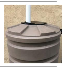
When installing the 3" pvc pipe or downspout be careful to keep the end of the pipe up above the screened basket under the lid. This gap will allow debris to flow out of the pipe and into the basket for removal later.
